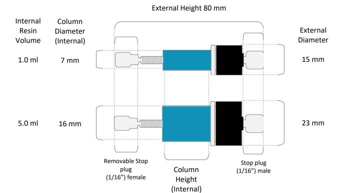
NOTE: HiFliQ FPLC columns are supplied with a moulded removable (1/16") female stop plug attached to the (1/16") male outlet port. Remove prior to use, reverse and use to seal the column for storage.
