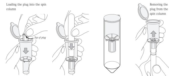
Place the plug into the spin column with the recessed end uppermost. Push the plug **FULLY** into the tapered end of the spin column using the plug insertion tool. It is now ready for preequilibration with binding buffer followed by centrifugation. After use, the plug is removed using the plug insertion tool.
