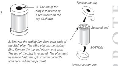
*Fig. 1. Schematic diagram of a Proteus Mini or Midi spin column plug.*
